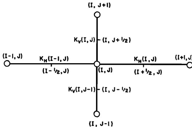
Fig. 5. Stencil for interior node used in development of finite-difference equation for two-dimensional, nonhomogeneous, anisotropic case.
