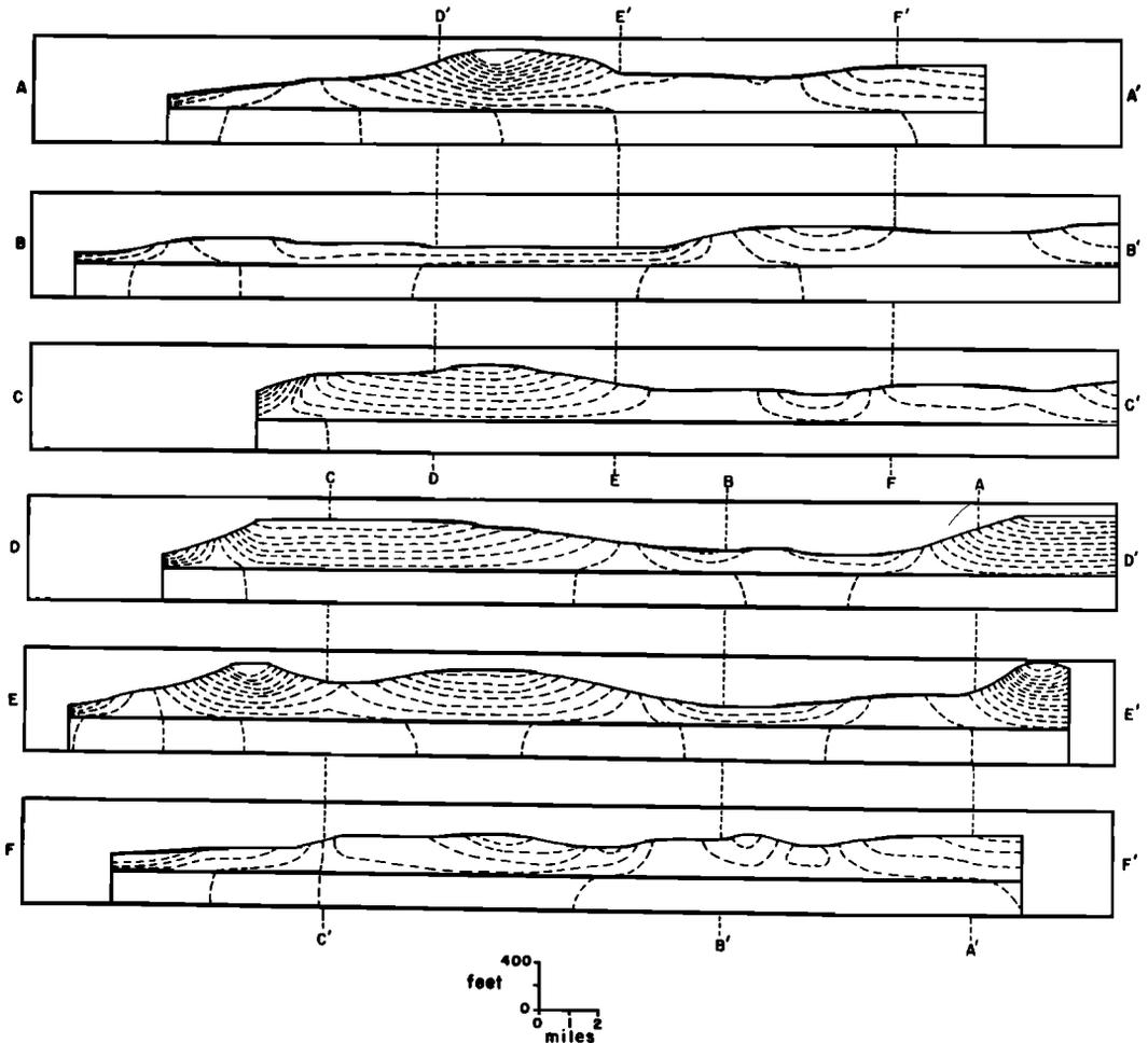
Fig. 9. Cross-sectional potential plots from three-dimensional model. Permeability of lower layer is 50 times that of upper layer.  $K_H = 20 K_V$  in both layers.
