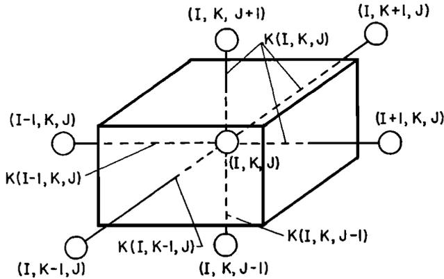
Fig. 6. Stencil for interior node in three-dimensional mesh for nonhomogeneous, isotropic medium.
