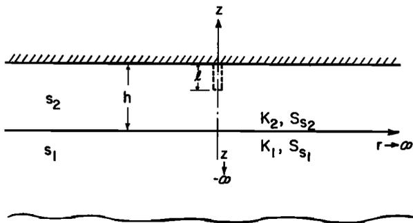
Fig. 1. Diagram of two-layer aquifer system with partially penetrating well.
