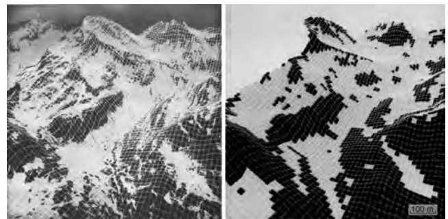
Figure 2. Observed snow cover pattern in (left) Kühtai, Tirol, and (right) model simulations on the same day. From Blöschl et al. [1991].
